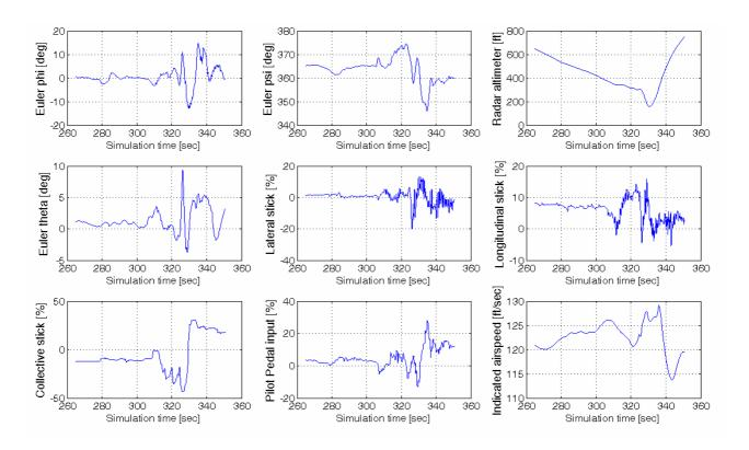
Figure 10 Encounter time history, 3° approach, 100% strength vortex at 300ft, GVE, pilot 1
