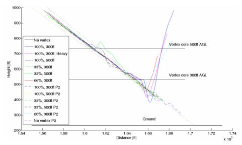
Figure 11 Height vs. Range plot for 3° GVE approaches
