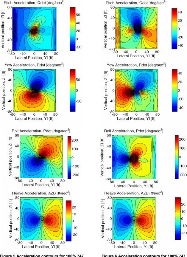
Figure 5 Acceleration contours for 100% 747 vortex (3° Glide slope, 0° Heading intercept, 70kts), (black dashed circle marks vortex core)
