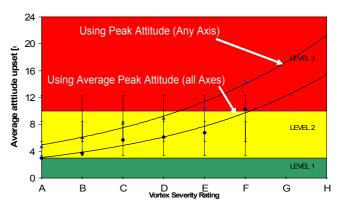
Figure 13 Vortex Severity Ratings versus averaged attitude upsets
