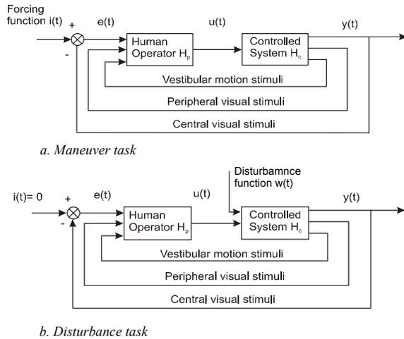
**Figure 3** - Differences in the influence of motion feedback in the maneuver task and the disturbance task
