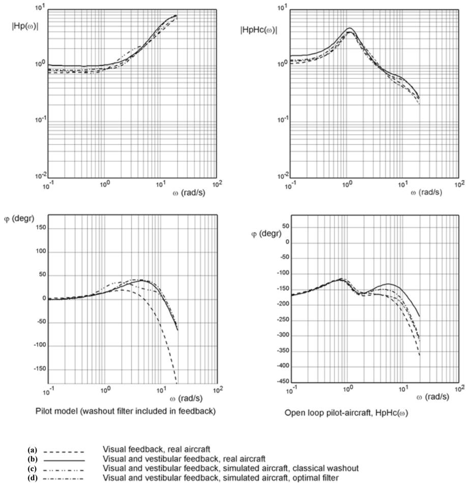
**Figure 5** - Bode plot of the pilot model and the pilot-aircraft open loop for the Wright Flyer in the disturbance task. Real aircraft with (a) visual and (b) visual and vestibular feedback, simulated aircraft with (c) classical washout and (d) optimal washout.
