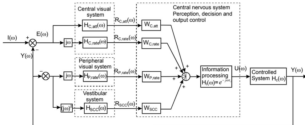
Figure 2 - Block diagram of the descriptive pilot model in the maneuver task.
