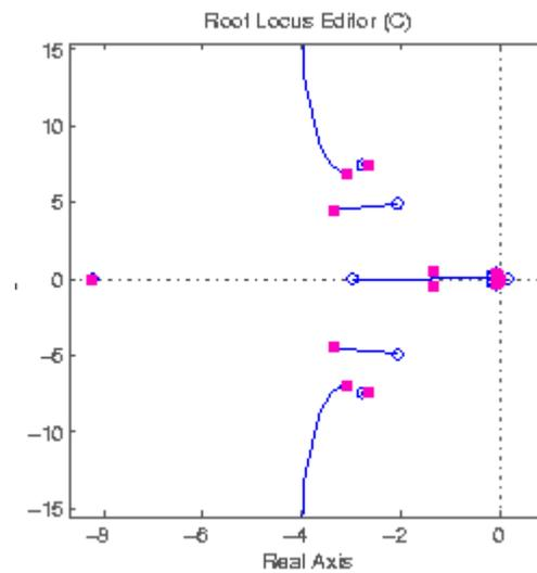
Figure 7 - Root loci with completed feedback gain matrix
