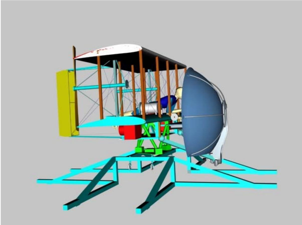
**Figure 8** – Concept of the Wright Flyer Simulator. Note the large frames allowing transportability of the system.
