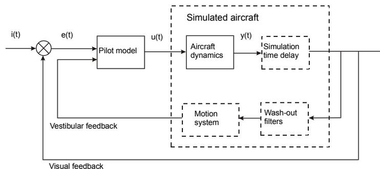
**Figure 4** – Closed-loop manual control in a simulation environment, showing most prominent contribution of simulation to the closed loop.
