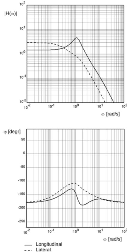
**Figure 1** – Longitudinal and Lateral Dynamics of the 1903 Wright Flyer.
