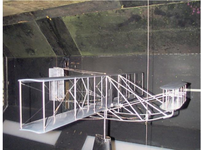
Figure A.1. 1/8th Scale 1905 Flyer Model in the Goldstein  $9 \times 7$ -ft Wind Tunnel.
