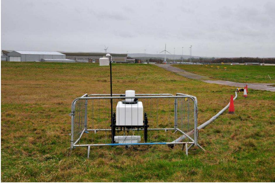
Figure 3.9: The on-site Galion LIDAR.
