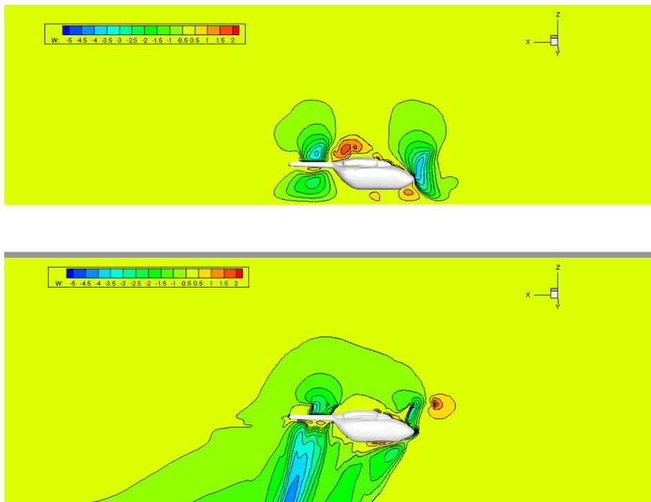
Figure 8.5: Downwash velocity contours around an approximate EC145 helicopter in IGE (0.75R) and OGE, hover-taxiing speed 20 kt.
