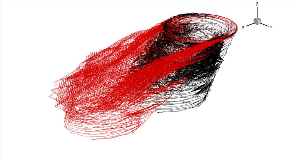
Figure 3.2: Dauphin tip vortex geometries predicted using the free wake model at  $\mu = 0.15$  (red lines) and  $\mu = 0.05$  (black lines).
