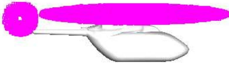
Figure 8.1: EC145 fuselage with main rotor and tail rotor actuator disks.
