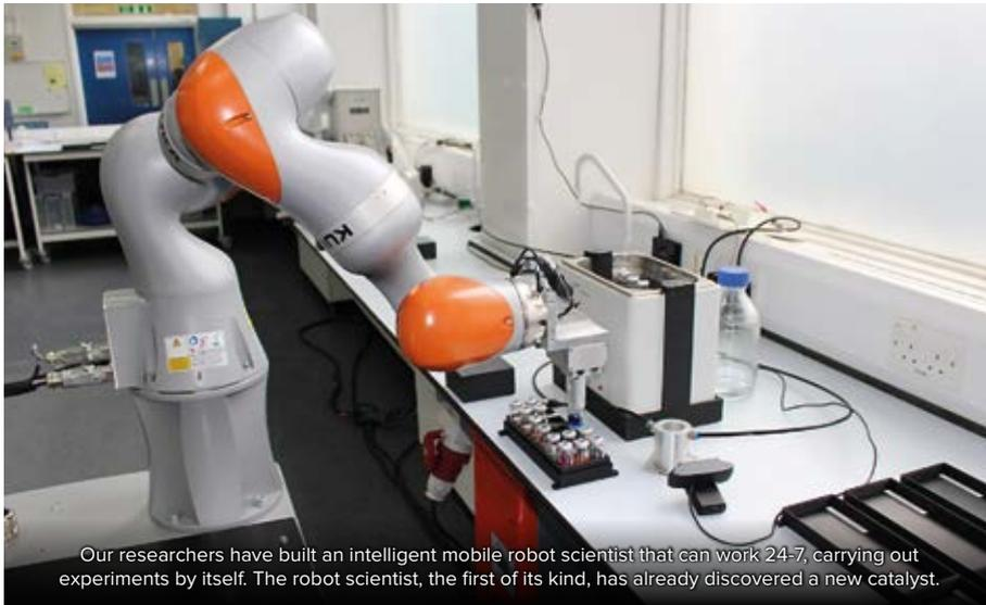
Our researchers have built an intelligent mobile robot scientist that can work 24-7, carrying out experiments by itself. The robot scientist, the first of its kind, has already discovered a new catalyst.
