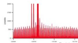
Measured longitudinal profile of heavy ion beam in the LHC with 500 ns bunch spacing. The main bunch arrives at  $\approx 18.060$  ns and is preceded by two satellites; ghost bunches spaced at 2.5 ns are present around the ring.
