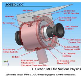
For the slow extraction from the SIS100 synchrotron the high-energy beam transfer-lines require diagnostic devices for the non-destructive measurement of ion currents down to the nA region. For this purpose, the installation of Cryogenic Current Comparators (CCC) is foreseen, offering a non-intercepting and absolute current measurement.
