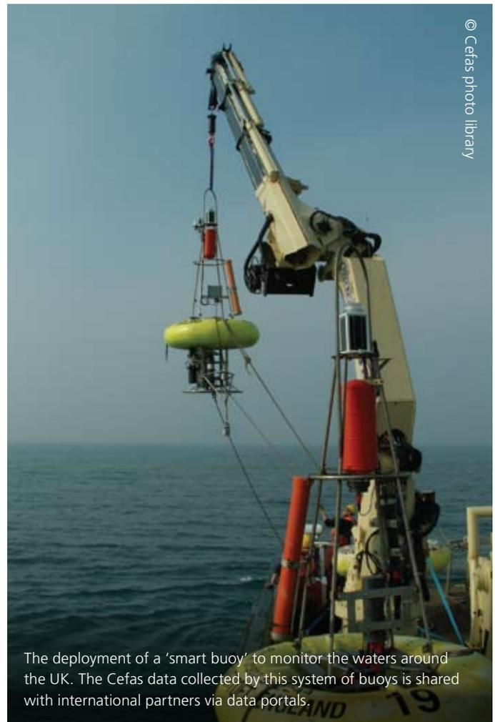
UK-designed 'smart buoys' provide rapid detection of environmental change in shelf sea waters with satellite-based data transmission.
