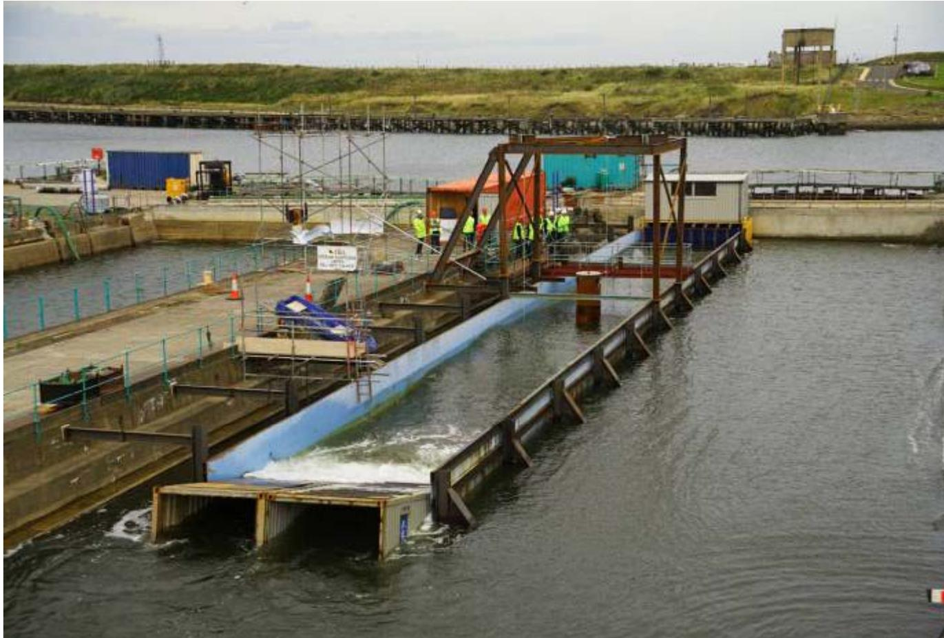
**1/10th scale tank testing 2005 – 2006, NaREC.**
