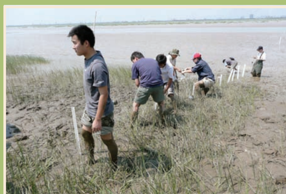
Figure 4: Sampling of sediments in the intertidal zone to establish the vertical zonation of forams and diatoms as a function of tidal inundation.
