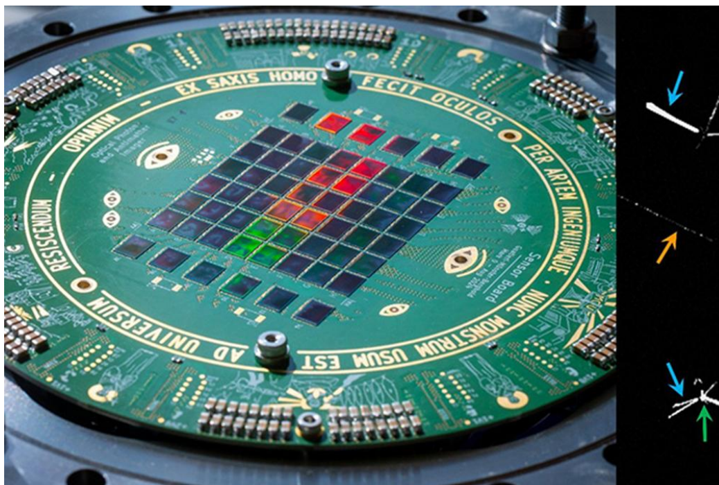
The Optical Photon and Antimatter Imager, integrating 60 sensors, and some examples of antiproton annihilations obtained with it. Credit: AEgIS/CERN.
