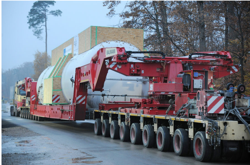
Delivery of the coldbox for the FAIR cryogenics facility.
