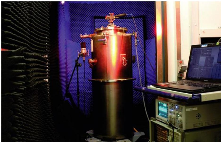
Prototype of the Cryogenic Current Monitor
