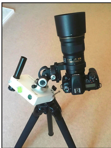
Figure 1. Nikon camera and lens on an iOptron SkyTracker (white box). The tracker rotates the camera at 1 rev/day and so, providing that the tracker is aligned parallel to the Earth's axis using the small polar alignment scope, the camera will follow the stars.
